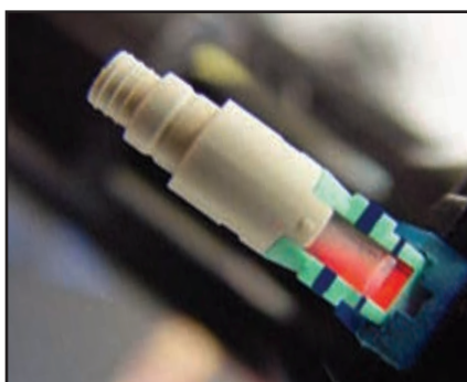
A light can be seen through the clear window on the connector body until a fiber has been properly terminated.
